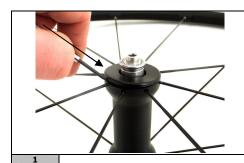
With a flat-bladed screwdriver remove the first protective cover. Make sure you do not damage the cover's locking teeth which would affect reassembling at a later stage.
