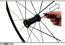
Remove the cone from the axle.
