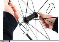
Insert the two 5mm hex wrenches inside the hexagons of the hub's body and tighten firmly. The right wrench (on the opposite side of the adjustment ring nut) remains fixed, the left wrench rotates clockwise.
