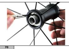
Check the cone is mates correctly into the bearing retaining ring.
