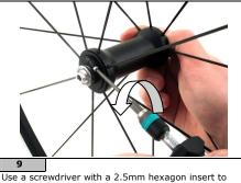
Use a screwdriver with a 2.5mm hexagon insert to loosen the screw of the adjustment ring nut.
