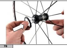
Inspect the dust covers. If they are damaged, replace them. Insert the cover with the larger internal diameter on the body of the hub on the adjustment ring nut side.
