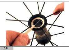
Remove the grease shield by using a small standard screwdriver. Repeat on the opposite side.
