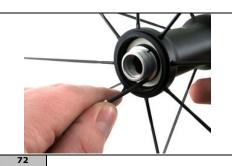
Manipulate it into position by using a small screwdriver. Push the adjustment cone in by pressing on various points of the circumference.
