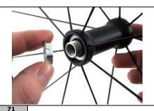
Insert the adjustment cone onto the axle mating into the cone from 69-70. The direction it should be inserted in. The larger diameter should face the outside of the hub's body.
