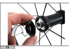
Inspect the adjustment ring nut. If it is damaged, replace it.
