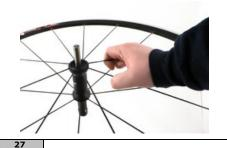
Use care not to glance off of the punch as damage can occur to the wheel.
