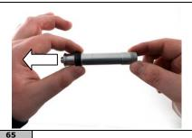
Ensure that the cone seats properly onto the corresponding cone shape on the axle.
