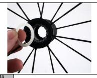
The black part of the grease seal should face the inside of the hub's body.
