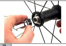
Remove the cone and the adjustment cone.
