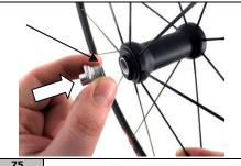
Inspect the axle end cap. If it is damaged, replace it.
