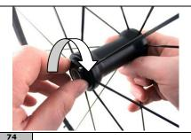
Install and tighten the adjustment ring nut clockwise and hold the axle while holding the axle stationary with your right hand.
