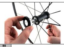
Insert the cover with the smaller internal diameter on the body of the hub on the side opposite to the adjustment ring nut.
