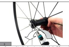
the tolerance of the axle movement with respect to the bearings a torque value with a range from 1.2 Nm (11 in lbs) to 3.0 Nm rolling in the cups and cones of the hub. To check whether the (27 in.lbs) set to conduct a 2.5 Nm (22 in.lbs) closure. adjustment is necessary, hold the rim with one hand, in with the other move the axle to identify if the tolerance is too loose or tight.
