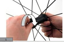
Holding the axle stationary, rotate the adjustment ring nut clockwise by about 1/8 of a turn.
