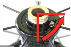
Keeping the pivot still, unscrew the ring by  $\frac{1}{4}$  of a turn (90°).
