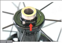
The ring is loose when the crack of the joint is visible.
