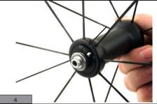
The indication that the adjustment ring nut will be loosened will be when the slot in the nut has a visible gap. Do not remove the screw from the adjustment ring nut.
