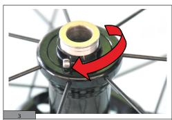
Keep the pivot on the other side still and screw in the ring until it stops.
