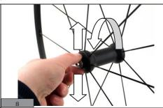
Check the movement of the axle when it rotates, if necessary repeat from point no. 2.
