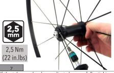
If the tolerance has been adjusted successfully, tighten the 2.5mm Allen screw with the torque wrench screwdriver set to **2.5 Nm (22 in.lbs)**. To reach the pre-defined torque, wait for the tool to indicate the proper torque.
