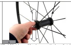
Check if the tolerance of the axle movement has been adjusted to satisfaction. If there is still unsatisfactory movement, carry out point no. 5 again.
