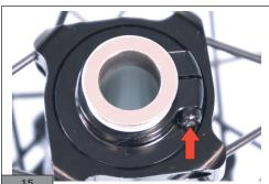
Lock the clearance recovery ring nut.
