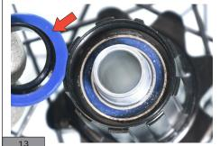
Install the seal and the spacer of the FW body.
