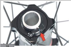
Keep the pivot on the other side still and screw in the ring until it stops.
