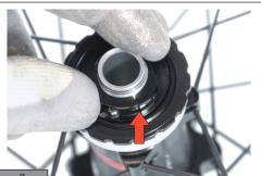
The ring nut is loose when the crack of the joint is visible.
