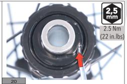
Tighten the screw (with a 2.5  $\,\mathrm{Nm}$  - 22 in.lbs tightening torque), using a torque screwdriver.
