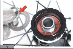
Remove the metal seal and the spacer.
