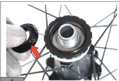
Working anti-clockwise, fully loosen the adjuster nut (holding the pivot stationary from the opposite side at the same time).
