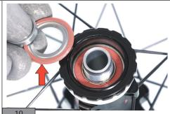
Install the DRP kit seal on the left hand side
