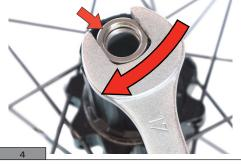
Unscrew the nut on the right using an 17 mm socket wrench.
