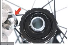
Remove the RH outer adapter from the pin.
