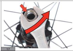
Screw in the nut on the right using a 17 mm wrench and tightening to a torque of 15 Nm.
