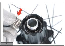
Remove the nut and the spacer.
