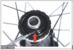
Loosen the screw which tightens the ring.
