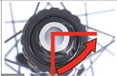
Keeping the pivot still, unscrew the ring by  $\frac{1}{4}$  of a turn (90°)
