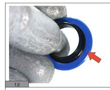
Install the seal on the spacer of the FW body. **Note**: from July 2018 the seal will be black.
