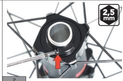
Ensure that the clearance recovery ring nut is tightened (screw tightened to 2.5 Nm) so that the ring nut does not turn.
