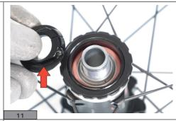
Install again the clearance recovery ring nut.
